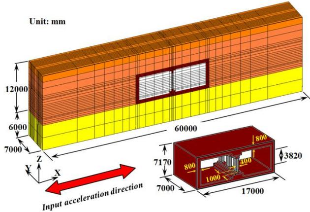
Fig. 8. 3D FEM mesh used for dynamic analysis in numerical tests
