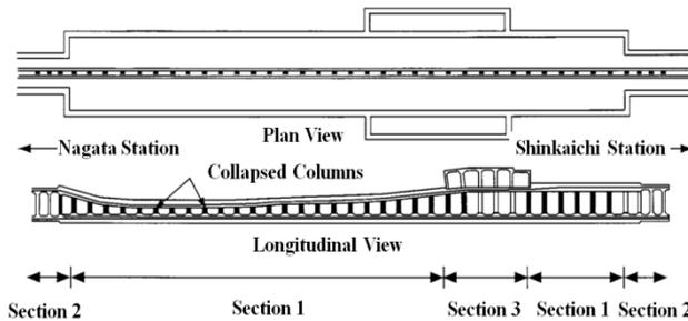
Fig. 1. Longitudinal damage patterns to the Daikai Station (adapted from Iida et al., 1996)
