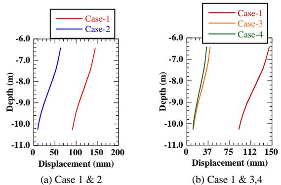
Fig. 14. Distribution of maximum horizontal displacement along height of column in Case-1, 2, 3 and 4
