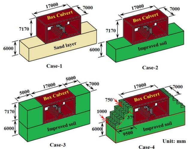
Fig. 11. Patterns ground improvement considered in 3D analyses
