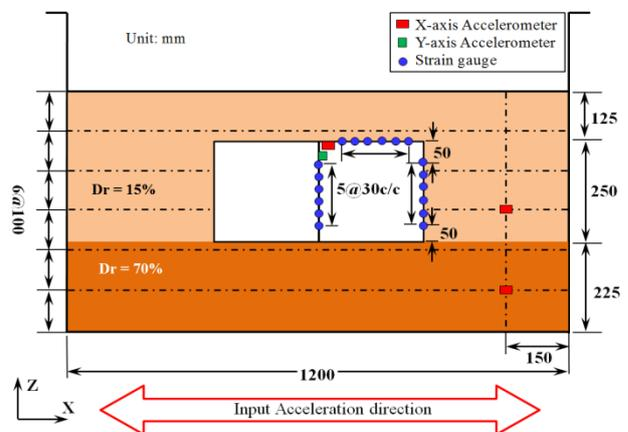
Fig. 4. Model box culvert, soil layers and measuring points
