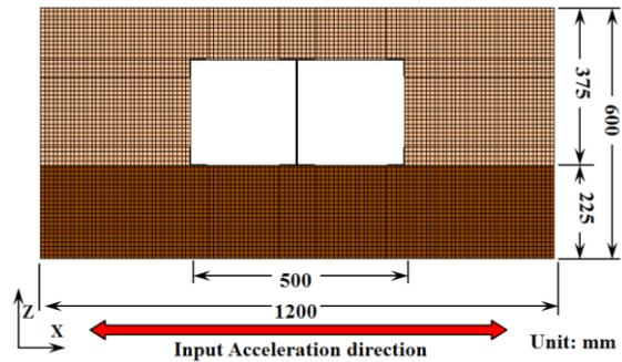
Fig. 6. 2D FEM mesh in model scale
