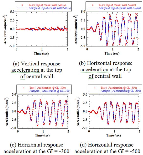
Fig. 7. Time history of acceleration from 2D analysis and shaking table test
