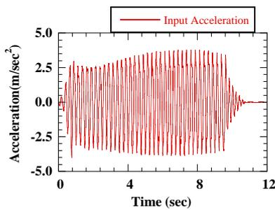
Fig. 5. Input acceleration in the shaking table test and 2D numerical analysis
