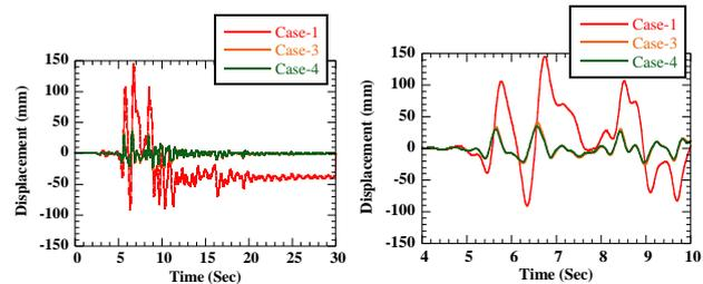
Fig. 13. Time history of horizontal displacement at top of central column in Case-1, 3 and 4
