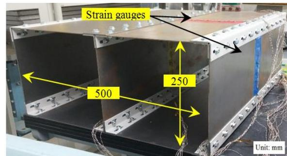
Fig. 3. Model box culvert
