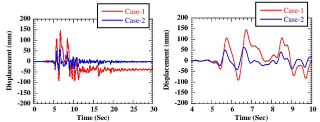
Fig. 12. Time history of horizontal displacement at top of central column in Case-1&2
