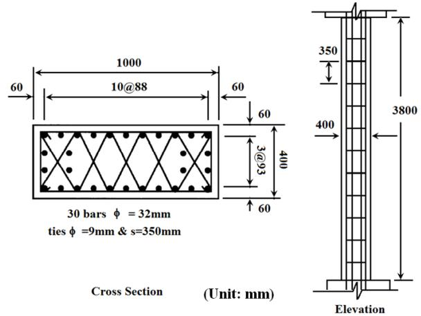
Fig. 9. Reinforcement of central column in Daikai station (Iida et al. 1996)
