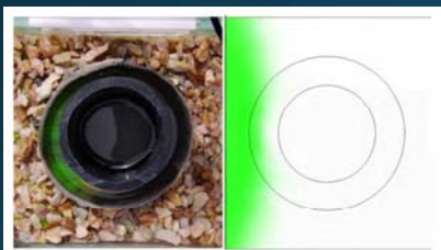
Figure 9: Plume of dye in laboratory setup # 1495 vs numerical result after ~20s.
